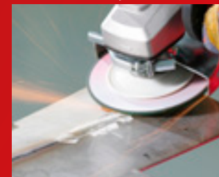
Remove and finishing of welding seams on stainless steel
