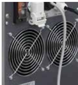
Detail of the control panel, with cooling fans and connection to the remote control of Fog Multi Ambiente module
