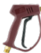
Spray gun ECO1, inlet M22x1,5 M, outlet G1/4" F, 280bar, 25l/min, 120°C
