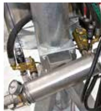
Detail of the AISI 303 stainless steel mesh filtering system
