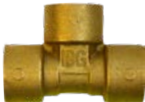
H.p. "T" connector, G3/8" F-F-F, pressure MAX 300bar, temperature 5-150°C
