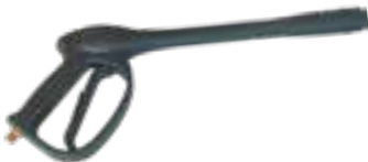
Spray gun with extension, 500mm, inlet G1/4" M, outlet M22x1,5 F, 220bar, 60°C
