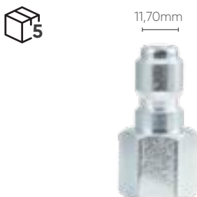
H.p. ball quick coupling, male, inlet Quick, outlet G1/4" F, 220bar, 30l/min, 90°C
