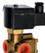
H.p. 2-way solenoid valve, 230V, 50/60Hz, 80bar, G1/2" F-F, NC
