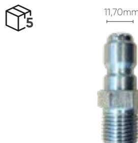
H.p. ball quick coupling, male, inlet Quick, outlet G1/4" M, 220bar, 30l/min, 90°C
