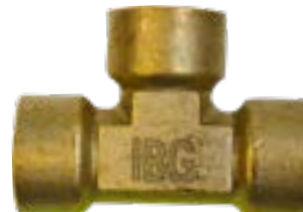
Brass h.p. "T" connector, G1/2" F-F-F, pressure MAX 300bar, temperature 5-150°C
