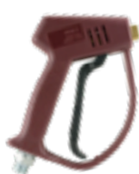
Spray gun ECO1, inlet G3/8" F, outlet G1/4" F, 280bar, 25l/min, 120°C
