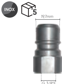
Male swivel ball quick coupling made of AISI 416 stainless steel, G3/8" F, 250bar
