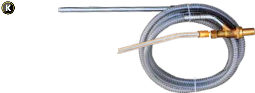
Professional sandblasting kit, inlet M18x1,5 F fitting Kärcher, 250bar, 40l/min. Complete with brass sandblast head with WIDIA insert, 4m suction hose and galvanised steel probe
