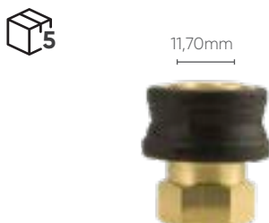
Ball nozzle holder with rubber guard. Made of brass, inlet G1/4" F, outlet Quick, 220bar, 30l/min, 90°C
