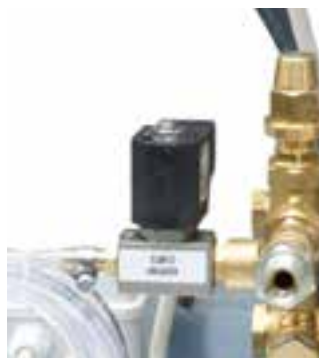
Detail of discharge solenoid valve and bypass valve
