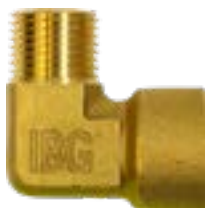
Brass h.p. elbow, G1/2" M-F, pressure MAX 300bar, temperature 5-150°C
