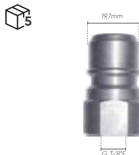
M swivel ball quick coupling male made of galvanised steel, G3/8" F, 250bar
