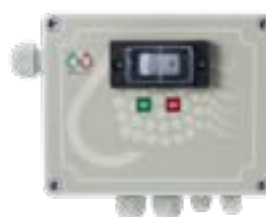
Electric panel Fog 60, complete with 7A thermal switch, 3m power supply cable, inlet and outlet solenoid valve power supply cable 230V Pressure switch connector and remote control connector.
