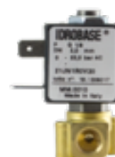
Solenoid valve brass body with plug, NC, G1/8" F-F, 230V, 25bar
