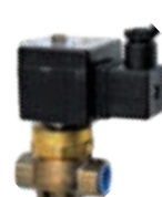
H.p. 2-way solenoid valve, 24V, 50/60Hz, 80bar, G3/8" F-F, NC. Stainless steel valve seat max 53l/min at 4bar
