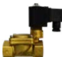
Solenoid valve brass body, NC, G3/4" F-F, 24V, 23bar, seal FKM, IP65
