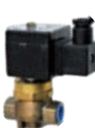
H.p. 2-way solenoid valve, 230V, 50/60Hz, 68bar, G3/8" F-F, NO. Stainless steel valve seat max 53l/min at 4bar
