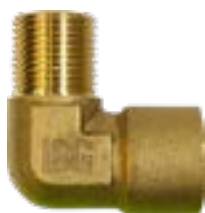
Brass h.p. elbow, G3/8" M-G1/4" F, pressure MAX 300bar, temperature 5-150°C
