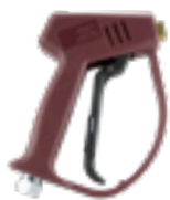
Spray gun ECO1, inlet G3/8" F, outlet G1/4" F, 280bar, 25l/min, 120°C
