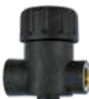
Inlet water filter, inlet G1/2" F, outlet G1/2" F, 10bar, 30l/min, 60°C
