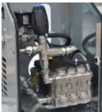
Pump head made and internal components made of AISI 316 stainless steel
