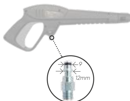
Quick coupling, G1/4" M for spray gun CDR.0447
