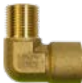
Brass h.p. elbow, G3/8" M-G1/4" F, pressure MAX 300bar, temperature 5-150°C Suitable for connecting the pressure gauge to the pump
