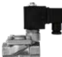
Solenoid valve SS body, NC, G1/2" F-F, 24V, 16bar, seal FKM, IP65
