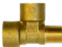
Brass h.p. "T" connector, G3/8" F-F-M, MAX pressure 300bar, temperature 5÷150°C
