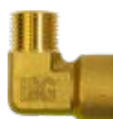
Brass h.p. elbow, G1/2" M-F, pressure MAX 300bar, temperature 5-150°C
