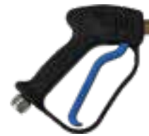
Aura weep gun, inlet G3/8" F, outlet G1/4" F, 210bar, 25l/min, 150°C
