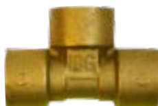
Brass h.p. "T" connector, G3/8" F-F-F, MAX pressure 300bar, temperature 5÷150°C
