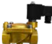
Solenoid valve brass body with plug, NC, G3/4" F-F, 230V, 23bar, seal FKM, IP65
