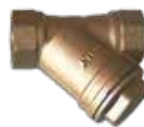
"Y" inlet water filter, made of brass, inlet G3/4" F, outlet G3/4" F
