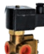
H.p. 2-way solenoid valve, 24V, 50/60Hz, 80bar, G1/2" F-F, NC
