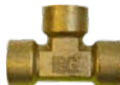
Brass h.p. "T" connector, G1/2" F-F-F, MAX pressure 300bar, temperatura 5÷150°C
